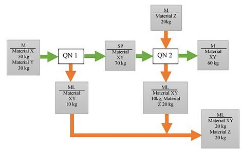
Figure 3. Material-energy flow model including semi-finished products
